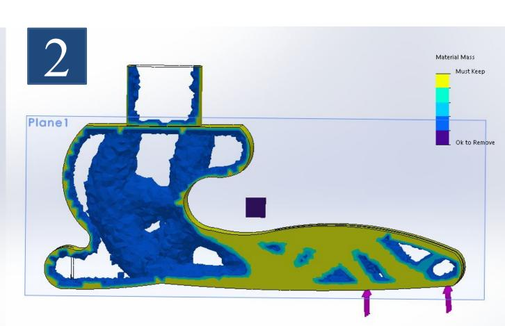
Solidworks software only utilizes the subtractive method of topology optimization, so a solid model of the original hollow cantilever split toe foot was created for topology optimization simulations.
